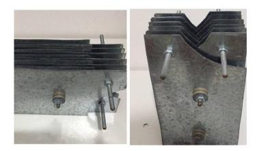
Figure 2 - Monopolar plates arrangement connected in parallel. Source: Own authorship.
