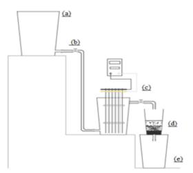
Figure 1 - Schematic drawing of electroflocculation prototype under continuous flow composed of: (a) feed tank (inlet), (b) valve, (c) electroflocculation reactor, (d) fixed bed filter and output. Source: Own authorship.
